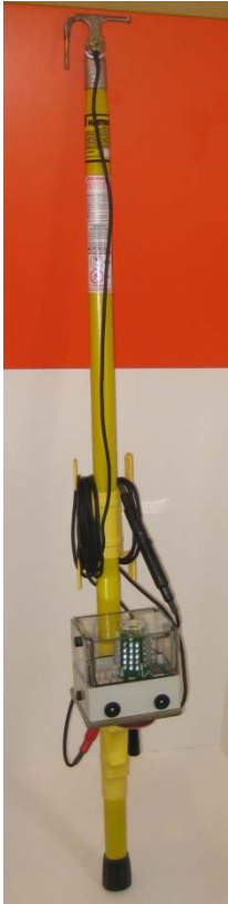
Unit is equipped with 1500VDC surge suppression and push button voltage meter
